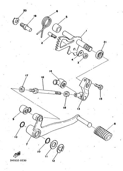
FIG. 23 SHIFT SHAFT.PEDAL
