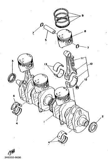
FIG. 3 CRANKSHAFT.PISTON
